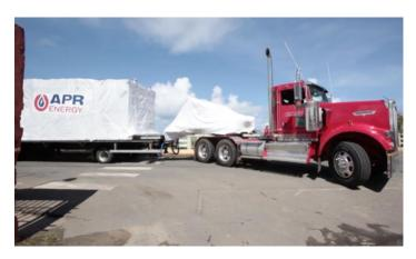
Corps of Engineers Oct. 12 to deliver two, 25 megawatt gas turbines to generate enough power to serve approximately 300,000 people. The company delivered the turbines the very next day and completed installation in a record 15 days, one of the fastest installations for a large-scale power project, according to APR.
